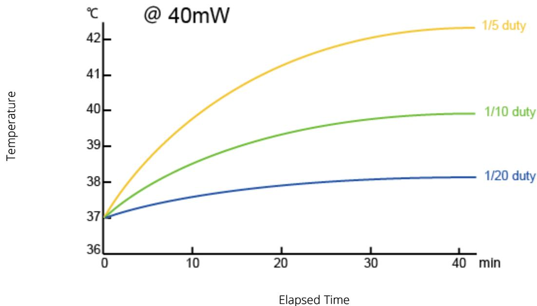
All the heat on the window surface will not reach the buffer inside the sample plate. The below graphs are simultaneous recordings of surface temperature and buffer temperature. Typically, after 30 ~ 40 minutes the buffer temperature will be equilibrated at 50 ~ 65% of surface temperature increase.
