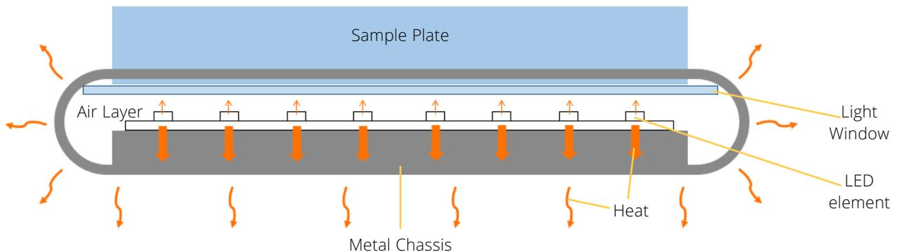
The surface temperature of the light window will be equilibrated at a certain temperature in 20 ~ 40 minutes. The below graphs are relationships between surface temperature and time at each light power:
