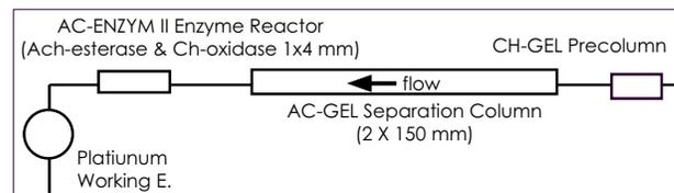
**Fig. 1 Flow diagram of HPLC columns and detection.** Enzyme immobilized column (reactor) and platinum working electrode can easily be used without chemical preparation such as enzyme modification of the working electrode.
