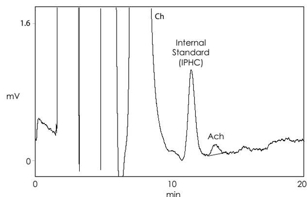
**Fig. 3 ACh analysis obtained from a 20 µl striatum microdialysis sample.** The ACh peak area corresponds to 10 fmol. This figure shows the basal condition following 3.5 hrs of aCSF perfusion without a cholinesterase inhibitor. The microdialysis probe used was Eicom CX-I-8-03, 3 mm active membrane length.
